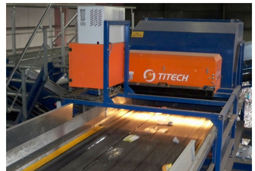
Photo of optical plastic sorter in action at J&B plant
